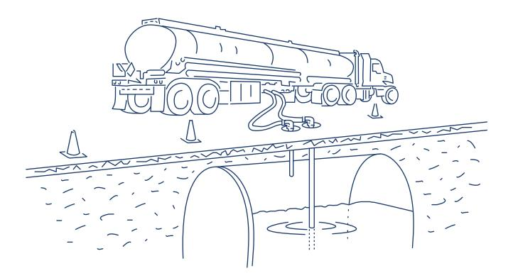
and preventing any contamination by liquid taken at a higher level. Some samplers will only sample to a depth of 14" from the bottom, so a tank owner should ensure the model purchased will pick up sediment or water directly off the bottom.
