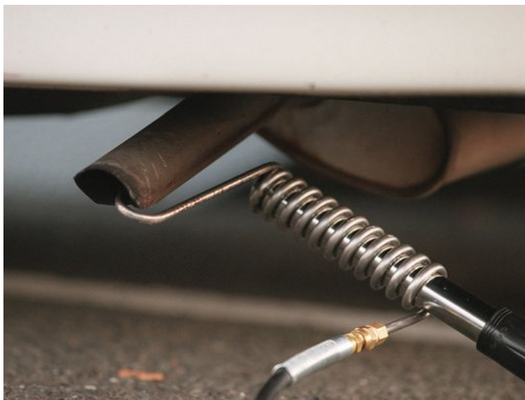
In this 1998 photo, SPX Corporations' exhibit with emissions sampler in tailpipe, Wednesday 12/2/98 at NJ DMV new emissions exhibition at National Guard Armory in Woodbridge. With wheels on a dynamometer, emissions will be tested with engine at running speed instead of idling. Mike Nixon/Staff (Photo: Digital Collections/IPTC)
